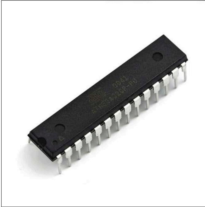
Figure 1-2: The Arduino's brain, an ATmega328 microcon- troller.
