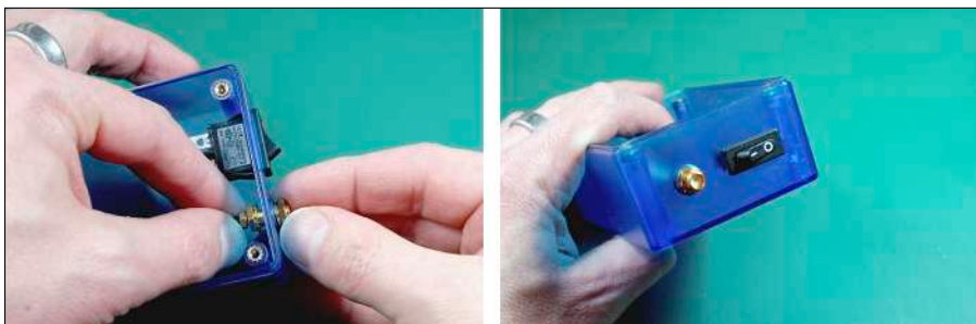
Figure 13-13: Mounting your power switch and pigtail SMA antenna adapter.
