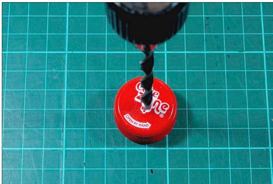
Figure 10-10: Drilling a hole for your supply line.
