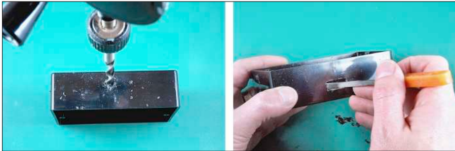
Figure 15-10: Drilling the hole for your power switch.
