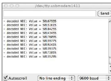
Figure 14-4: Example output of remote con- trol codes.
