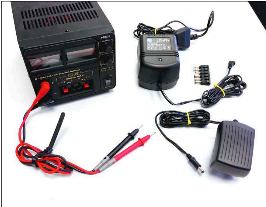
Figure 2-4: A bench power supply, a compact 12V trans- former, and a wall trans- former or “wall wart.”
