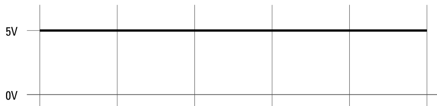
Figure 5-4: Using pulse-width modulation to change how long a digital pin is on or off. The vertical lines represent regular time intervals, usually 700 cycles per second.
