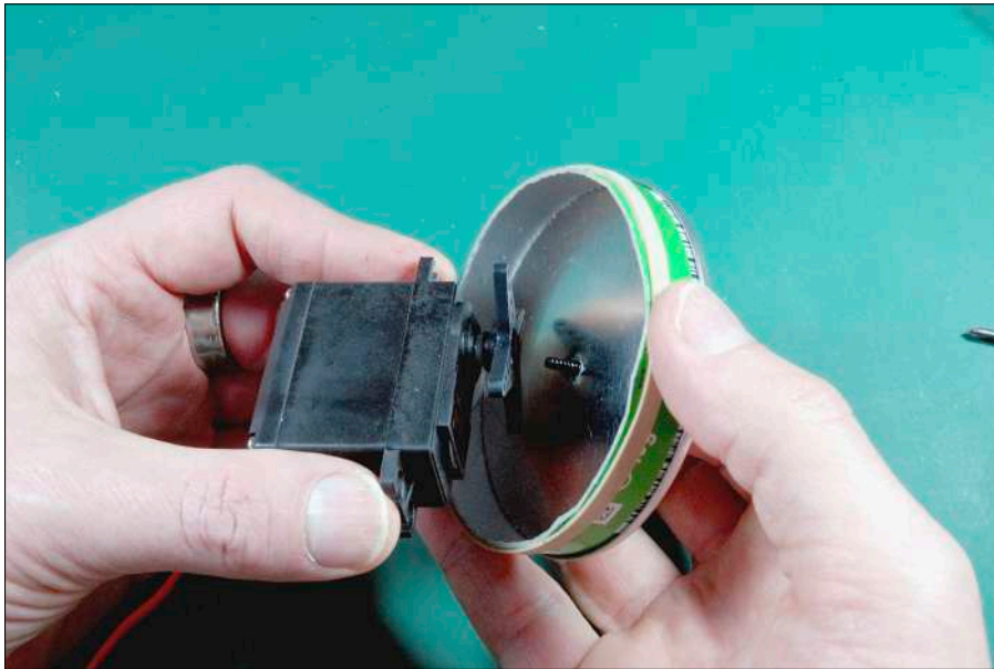
Figure 14-12: Mounting your wheels to the servo motors.
