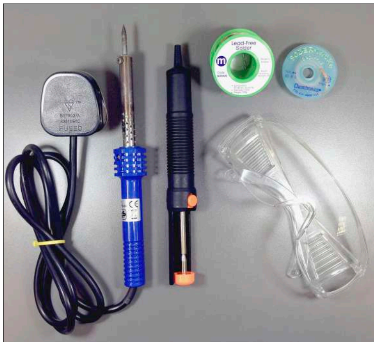
Figure 2-6: An entry-level soldering iron and essential accessories.
