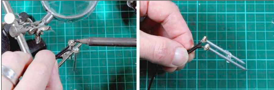
Figure 10-3: Soldering wires to your probe.
