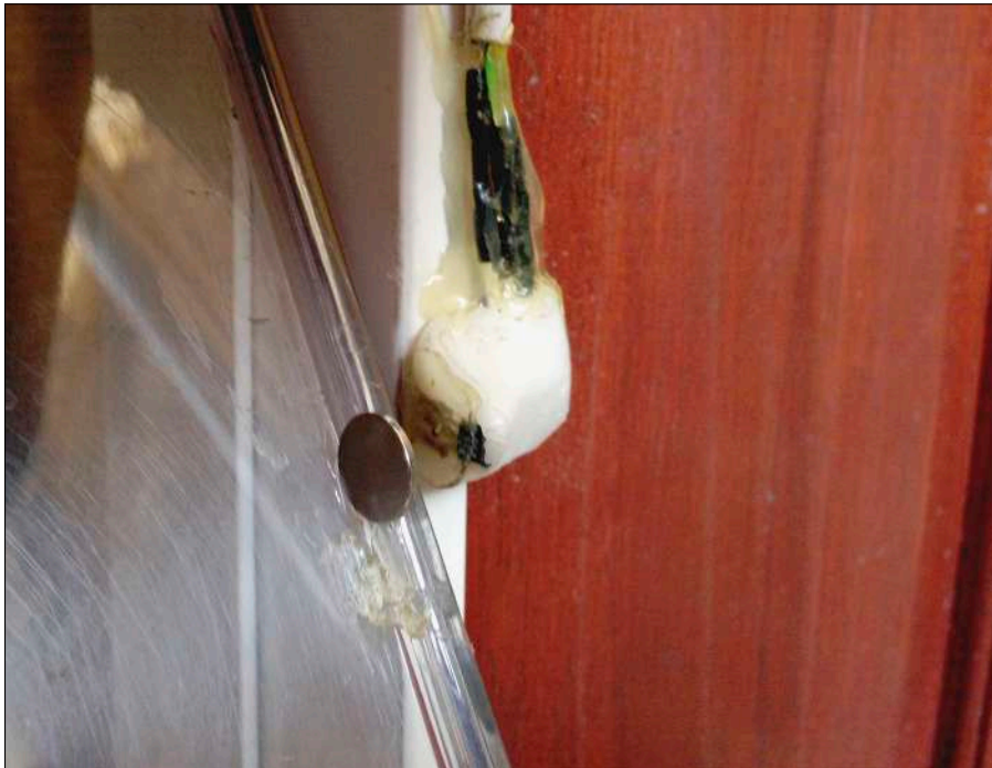
Figure 11-10: Mounting your sen- sors and magnets.
